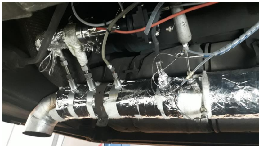
Horiba flowmeter and Pegasor attached to the city bus exhaust duct
