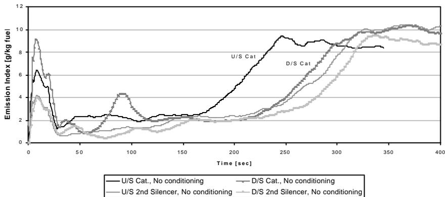
*DEPOSITION AND REENTRAINMENT ALONG THE EXHAUST SYSTEM AT THE NEW CONDITIONS TESTED*
