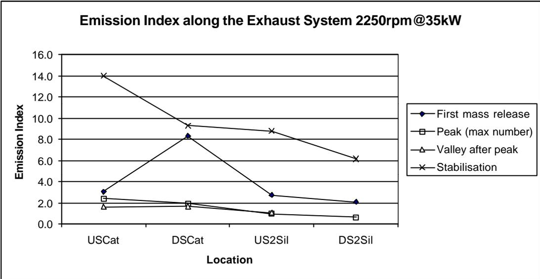
In the valley following the peak-by-number event, smaller changes in number concentration and mass were observed through the catalyst and the first silencer, and there was some evidence of particle growing through the catalyst and some deposition of particles through the first silencer.
