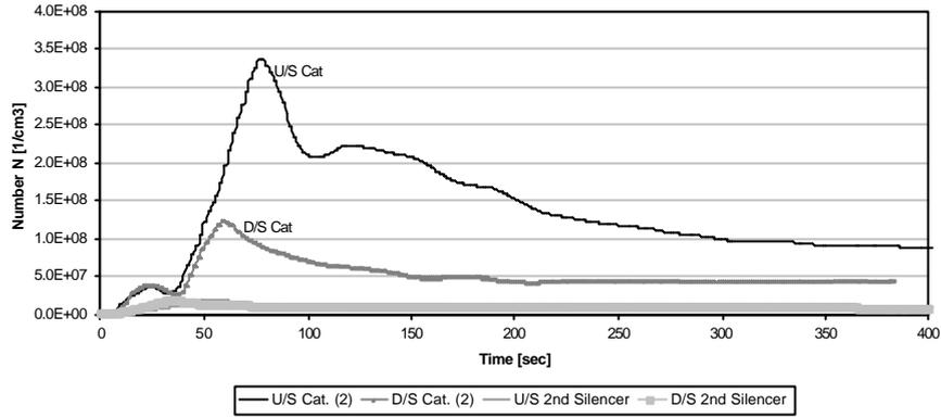
Emission Index Concentration during Cold Start, 3500rpm@15kW
