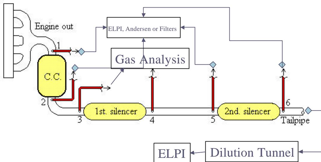
Engine: Ford 1.8L IDI Turbocharged Intercooled Diesel Engine. Exhaust system identical to the one installed in its commercial version.
