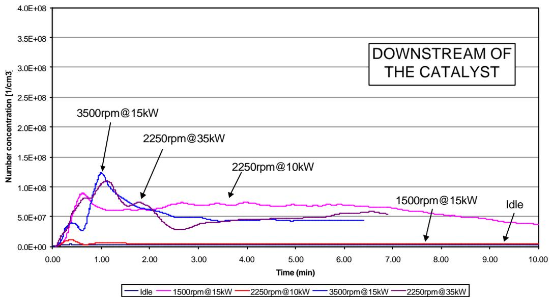
Total Particle Number Concentration during Cold Start, 3500rpm@15kW
