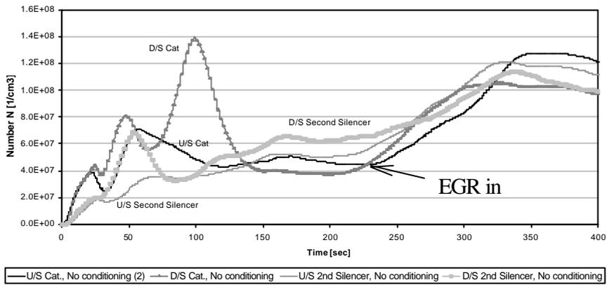
Emission Index Concentration during Cold Start, 2250rpm@35kW
