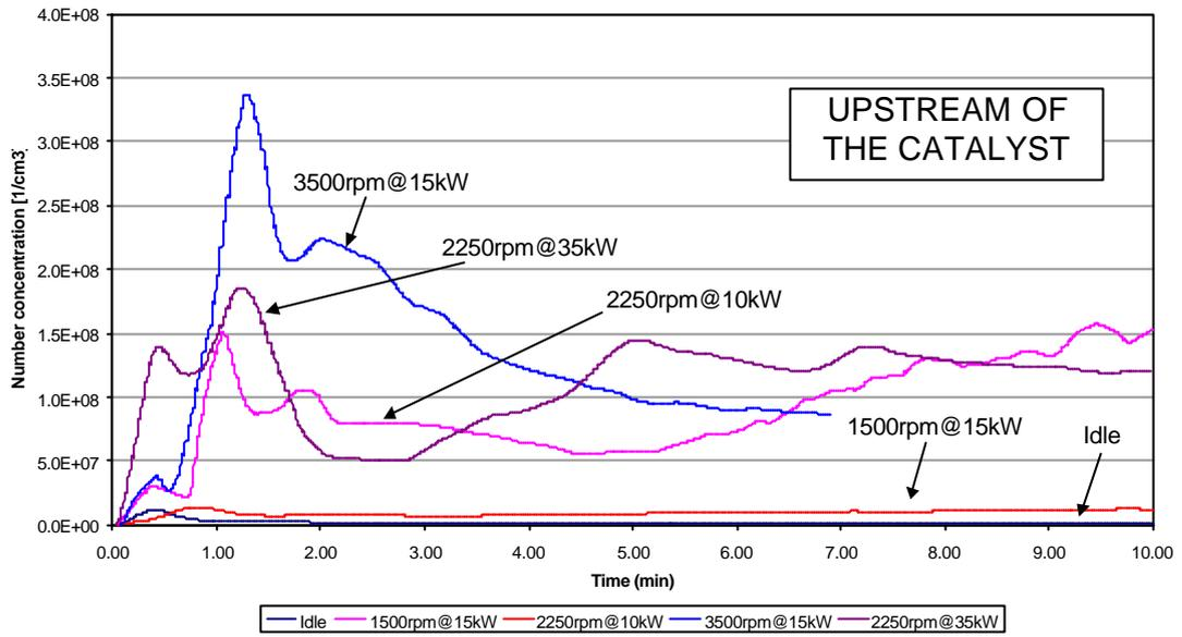
Compared to previous results, number concentration emissions at 2250rpm@35kW upstream of the catalyst resulted comparable to those at the same speed but 10kW power, whereas it was much higher when the speed was increased to 3500rpm keeping power at a medium level, 15kW. Downstream of the catalyst, number concentration levels at both high speed and high load conditions were comparable to those at 2250rpm@10kW.
