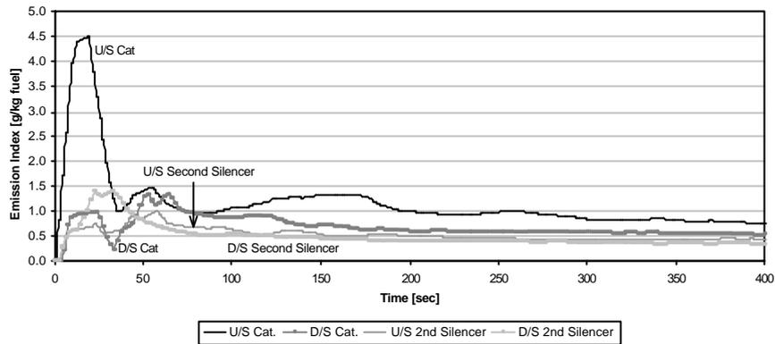
Total Particle Number Concentration during Cold Start, 2250rpm@35kW
