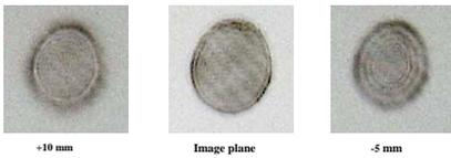
A webcam is used to investigate laser cross beam in the probe volume. We report single shot digital images of the cross beam taken in the image plane and away from this.
