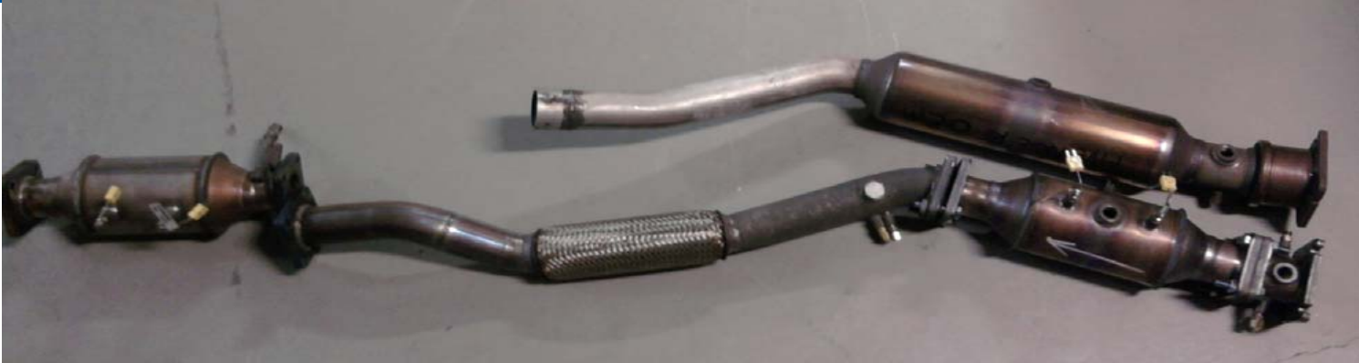
SULEV20 Performance Achievable with Efficient Precious Metal Placement in a Close-Coupled, Multi-Substrate Converter
