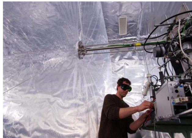
Smog chamber study on secondary aerosol formation
