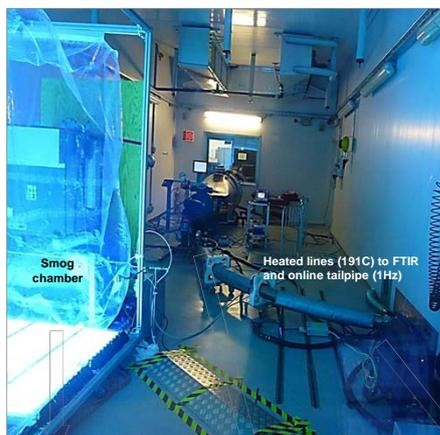
**Vehicle Emission Lab (VELA1)** at JRC. A 2-s and a 4-s moped are tested on legislated driving cycles (chassis-dyno) with controlled ambient conditions. Primary gaseous and particulate emissions are measured at the tailpipe and in dilution tunnel. Tailpipe exhaust is also injected in a photochemical aerosol **mobile smog-chamber** and Secondary Aerosol is characterized.
