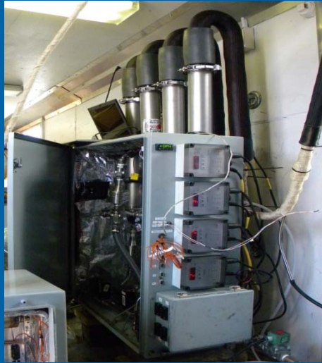
WVU Hi-Vol Thermodenuder Sampling System (WVU-HVTSS)
