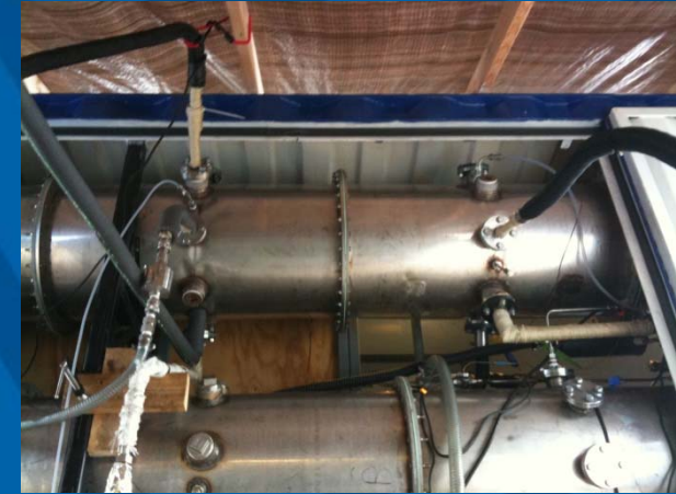
Clean tunnel CVS sampling plane
