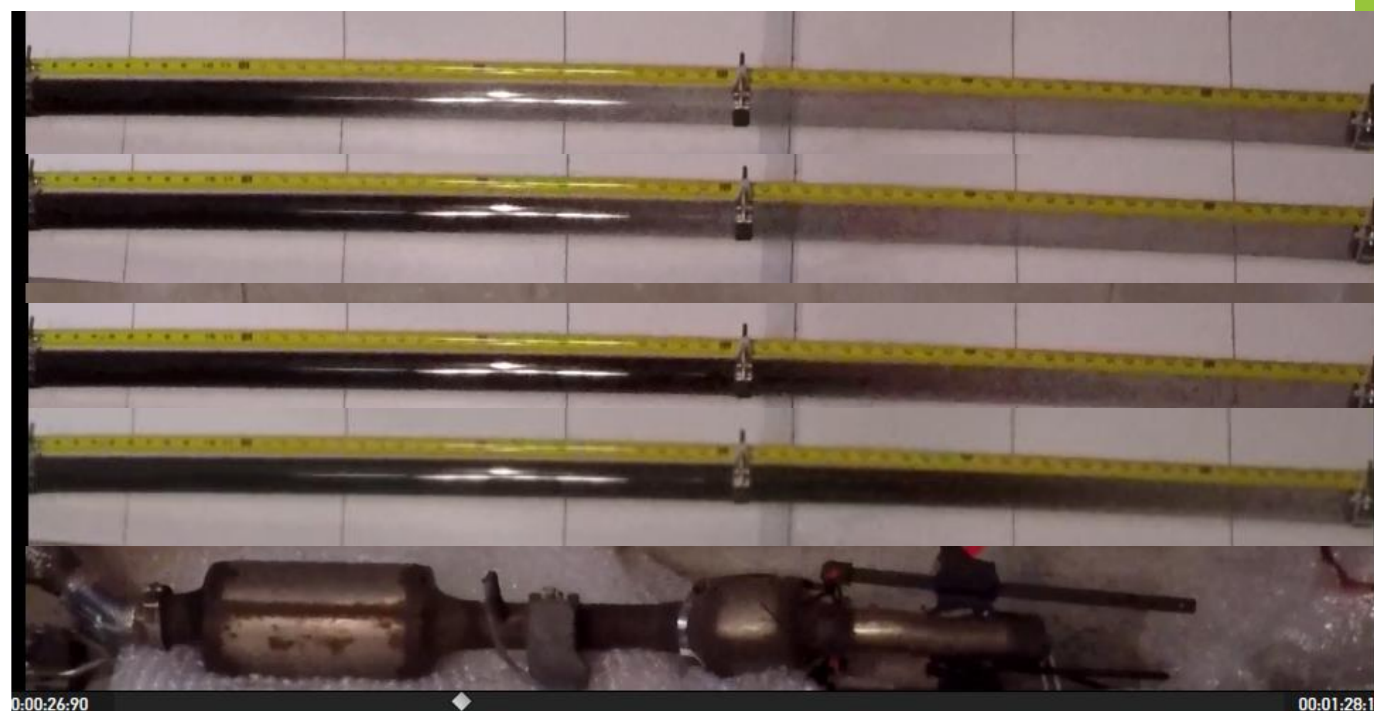
CPR Bench Test with Full System - sequential frames Regeneration @ 240 Frames/sec >160 km/hr Regeneration Exit Velocity
