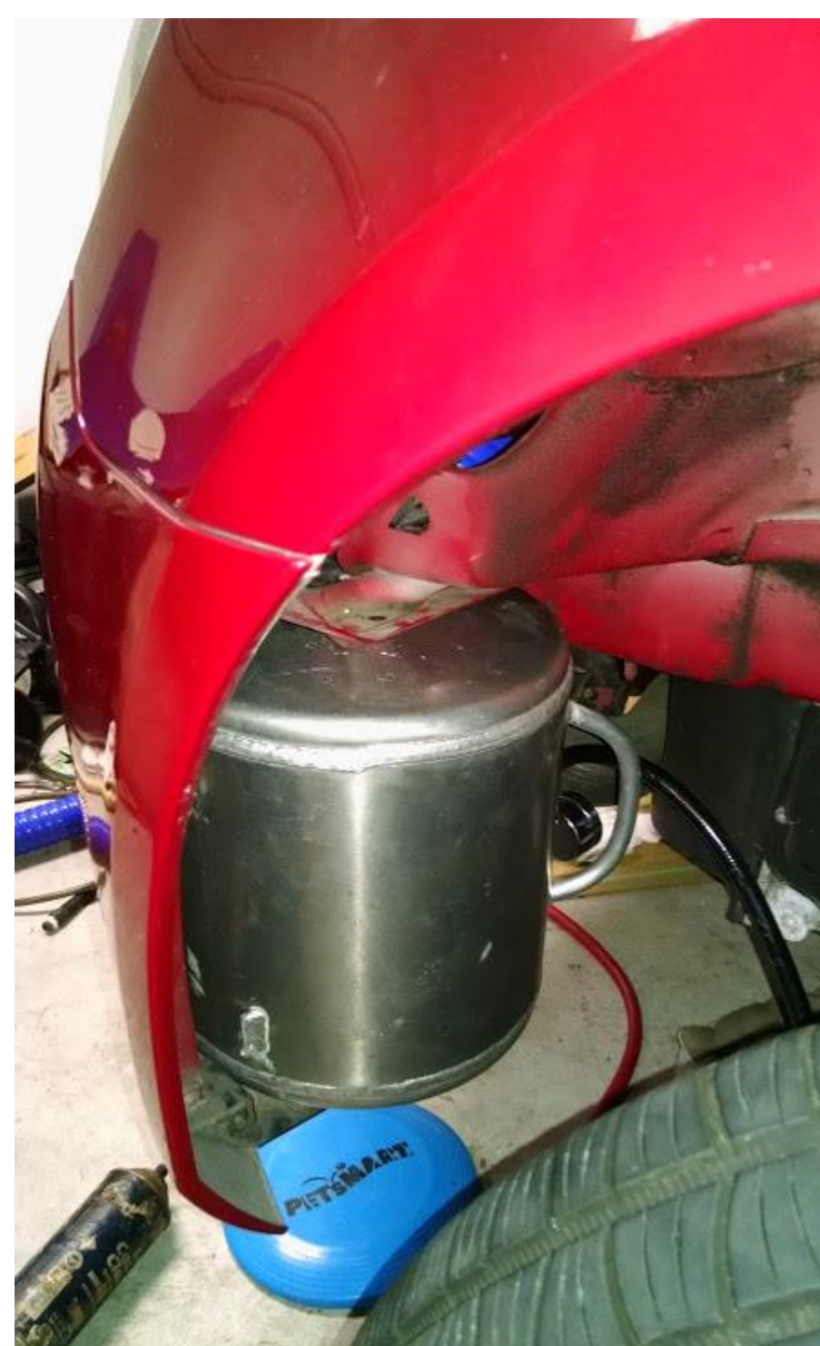
10.4 Liter Storage Tank Packaged within Front Fender
