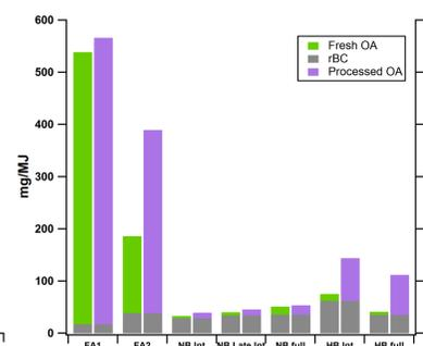
Figure 6. PM1 mass emission factors divided into refractory BC as derived from the SP-AMS data. Fresh Organic Aerosol (OA) and Processed OA (PAM reactor: 3\*10^8 cm-3h). Denotations as in Fig. 5.
