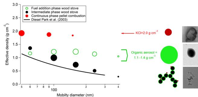
Figure 3. Effective densities derived from tandem mobility-mass measurements of wood stove and pellet boiler emissions. Comparison with TEM (right)
