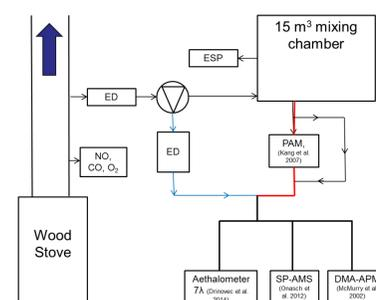
Figure 8. Schematic of the set-up used to characterise fresh and processed biomass combustion emissions.
