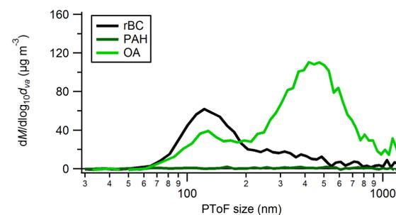
Figure 4. Size-resolved analysis with the SP-AMS, illustrating the separation of tar-balls and soot aggregates from a NB full cycle
