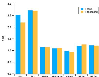
Figure 5. Absorption Ångström Exponents (AAE) derived from aethalometer (AE33) data for fresh aerosol and aerosol processed in the PAM reactor. FA: fuel addition phase, Int: Intermediate Flaming phase, NB: Nominal burn rate and HB: High burn rate. (Martinsson et al. 2015)
