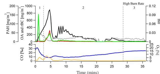
Figure 2. Time-resolved emissions measured with the SP-AMS of a high burn rate batch in the wood stove. The batch was initiated by adding fuel on glowing embers. 1. Fuel Addition, 2. Flaming (intermediate), 3. Burnout
