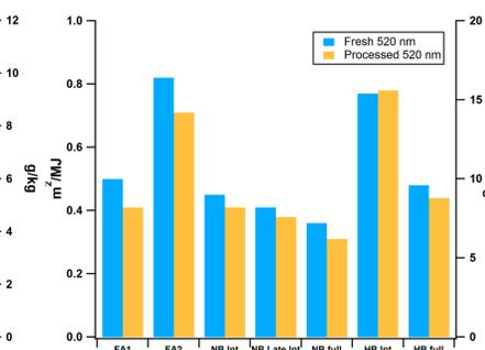
Figure 7. Light Absorbing Carbon (LAC) given as emission factors at 520 nm assessed from the aethalometer (AE33) data for fresh aerosol and aerosol processed in the PAM reactor. Denotations as in Fig. 5.
