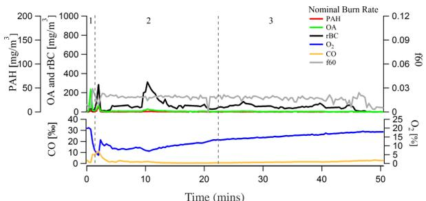
Figure 1. Time-resolved emissions measured with the SP-AMS of a nominal burn rate batch in the wood stove. The batch was initiated by adding fuel on glowing embers. 1. Fuel Addition, 2. Flaming (intermediate), 3. Burnout
