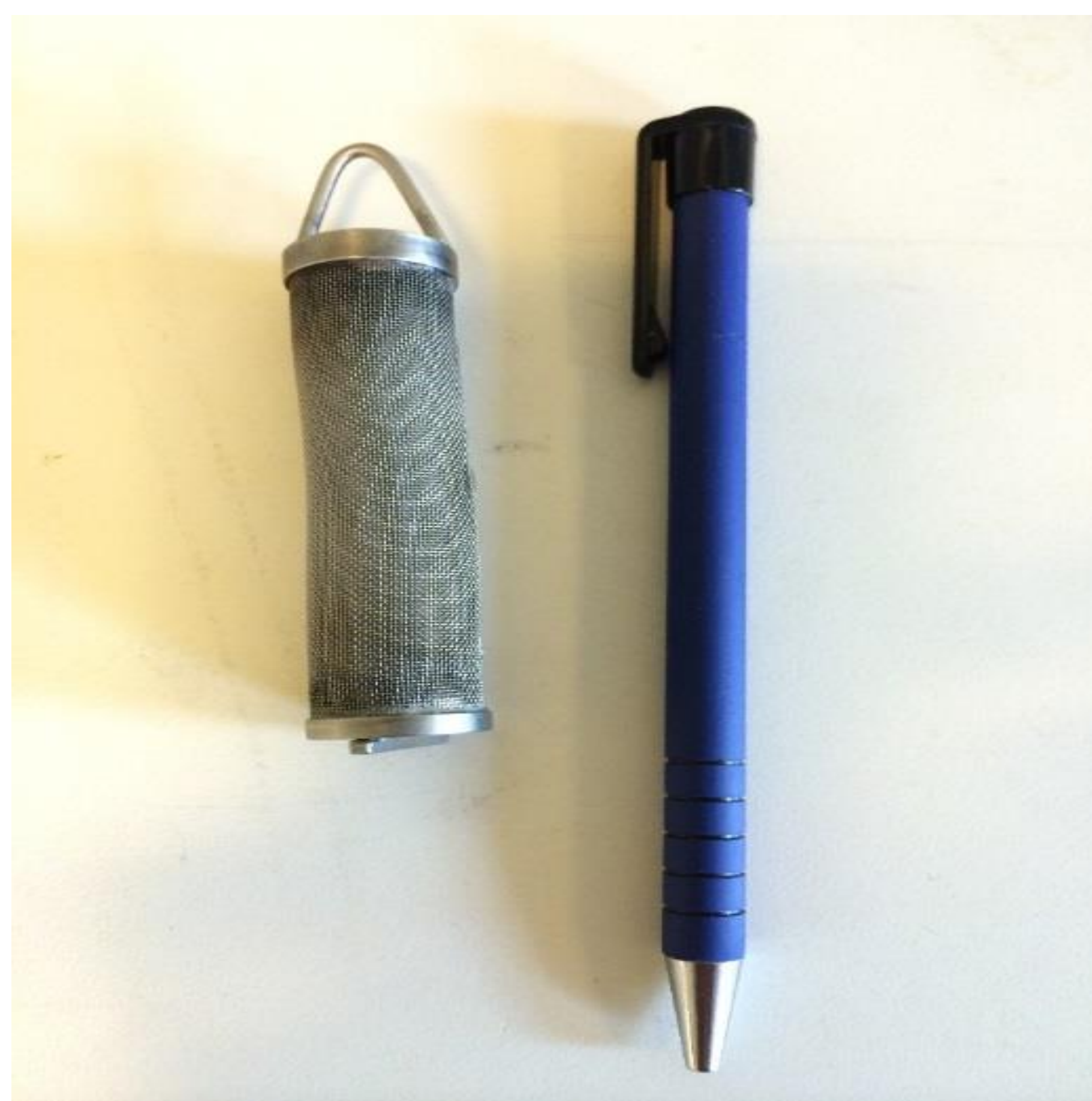
Adsorption sampler for powder materials.
