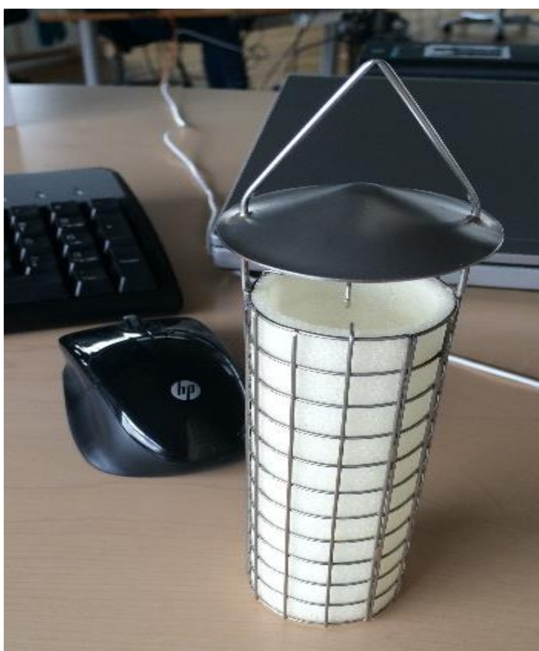
One of two designs of the adsorption sampler.
