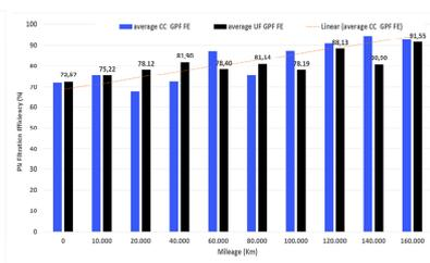
Fig. 3. PN GPF filtration efficiency (FE) versus mileage over the "average customer cycle" on road for UF & CC GPF
