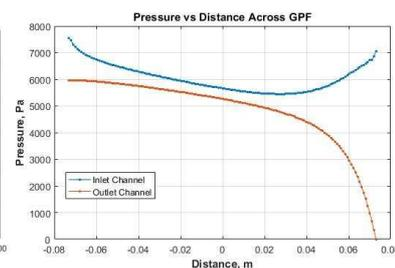
Fig. 7. Pressure distribution along GPF simulated channels, measured at centerlines.
