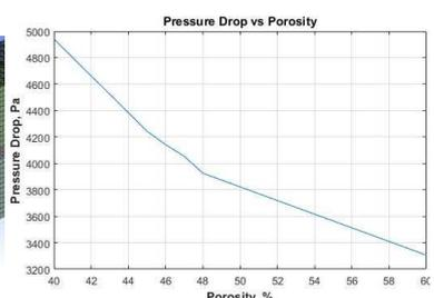
Fig. 5. Pressure drop across the GPF as function of filter porosity
