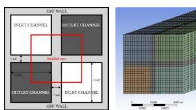
Fig. 4. GPF section geometry and mesh
