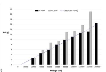
Fig. 2. Ash accumulated versus mileage up to 200,000 km for the UF and the CC GPF case.
