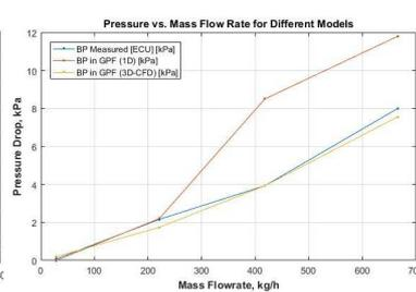
Fig. 6. Comparison 1D model vs 3D CFD model and ECU BP values for a clean CC GPF case (no soot no ash).
