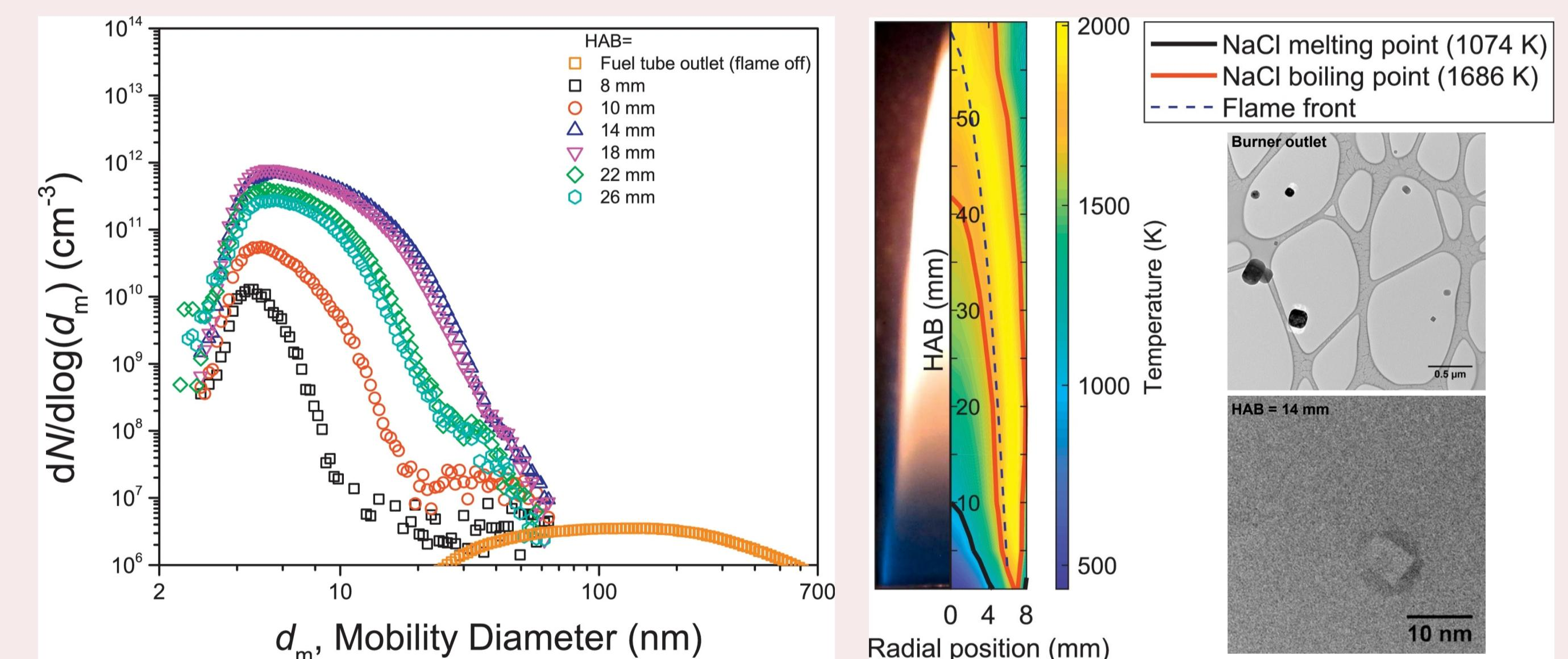
Fig. 4. Size distribution and TEM images of particles from methane-NaCl flame from burner outlet to HAB = 14 mm. The contour plot shows the temperature of the methane-NaCl flame.
