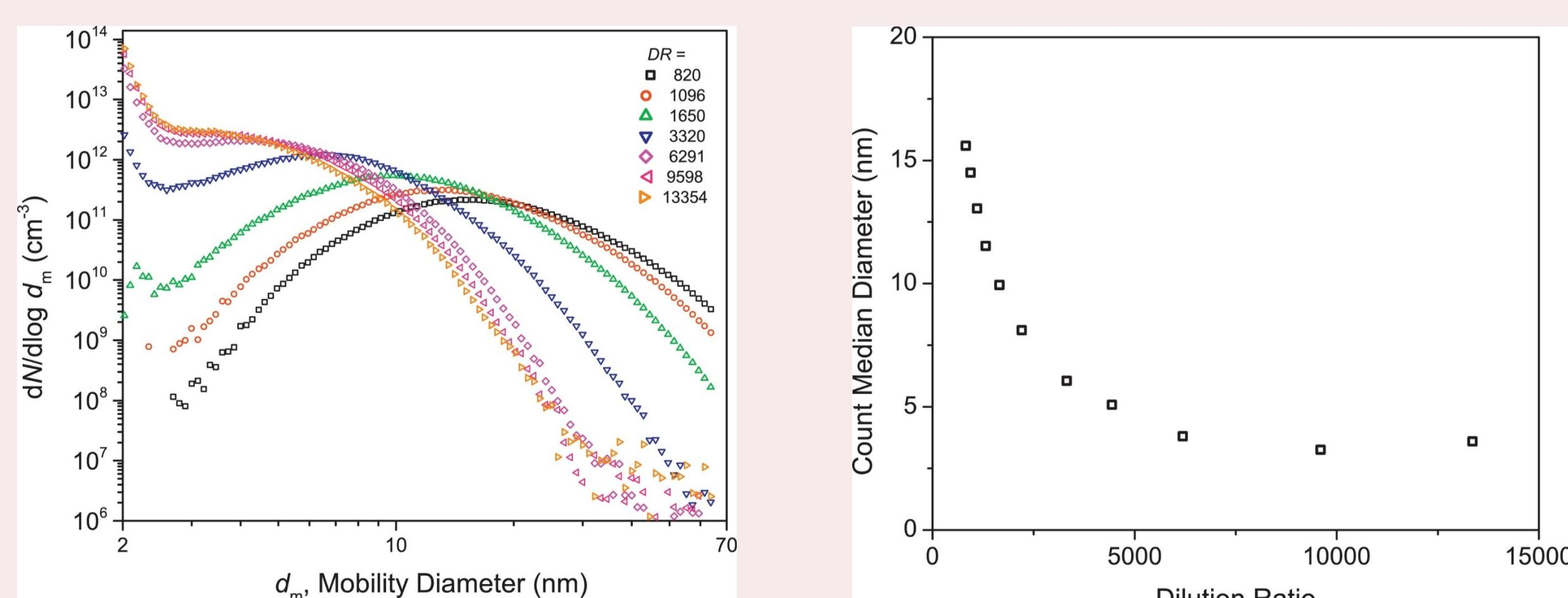
Fig. 2. Variations of particle size distribution and particle median diameter as a function of dilution ratio for HAB = 38 mm
