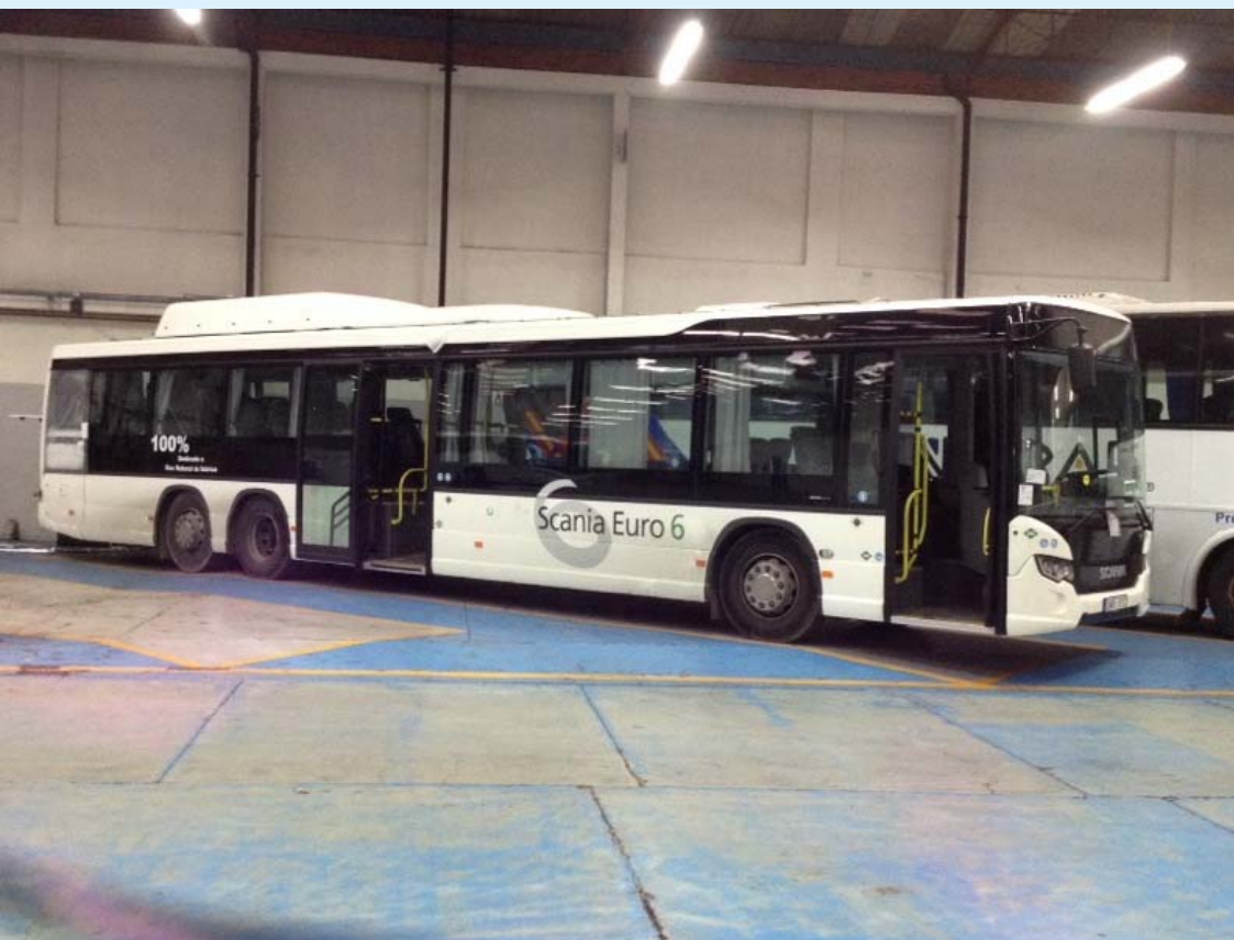
SCANIA K340 – Compressed Natural Gas (CNG) Engine Reference: OC09 102/250 kW (340 HP) - Stoichiometric
