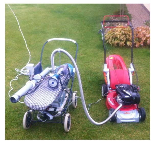
Sampling ("CVS") mode: • PEMS measuring diluted exhaust
