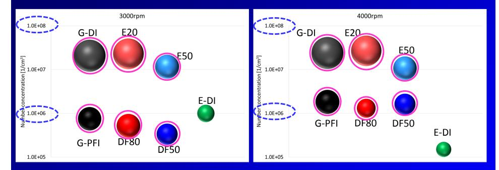
DF80: 80% gasoline (PFI) 20% ethanol (DI) E20: 80% gasoline (DI) 20% ethanol (DI)
