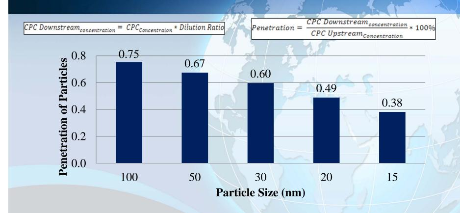
Highest losses in Primary section – largely thermophoretic losses.
