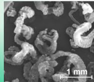
Fig. 2 – Expanded graphite
