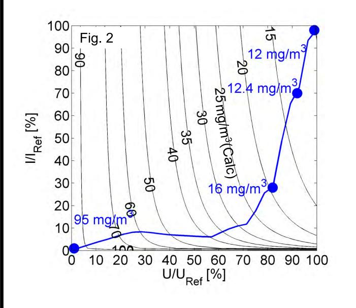
**ESP Operating Points:** Due to the lack of a reliable and affordable sensor to continuously measure PM emissions from biomass combustion, ESP operation has to be monitored depending on applied voltage and current.
