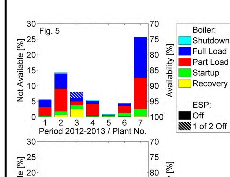
Fig. 5 allocates phases with unavailable ESP to boiler operating modes.
