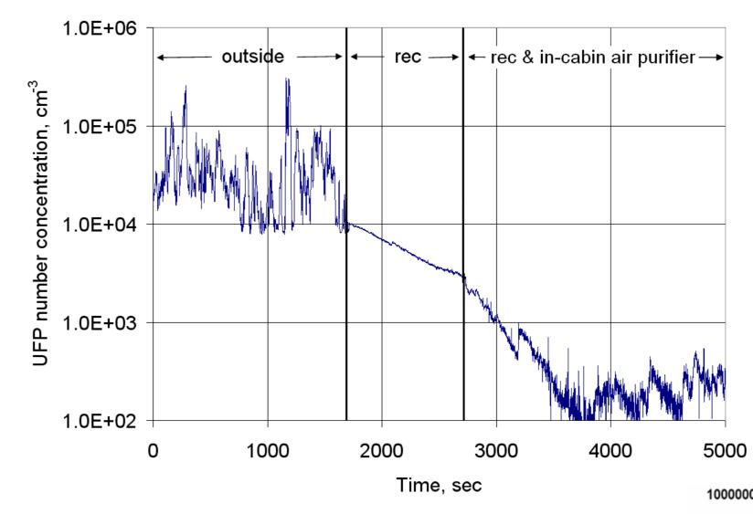
UFP concentration outside and inside the cabin, with AC in recirculating mode and after starting the-retrofit HEPA filter
