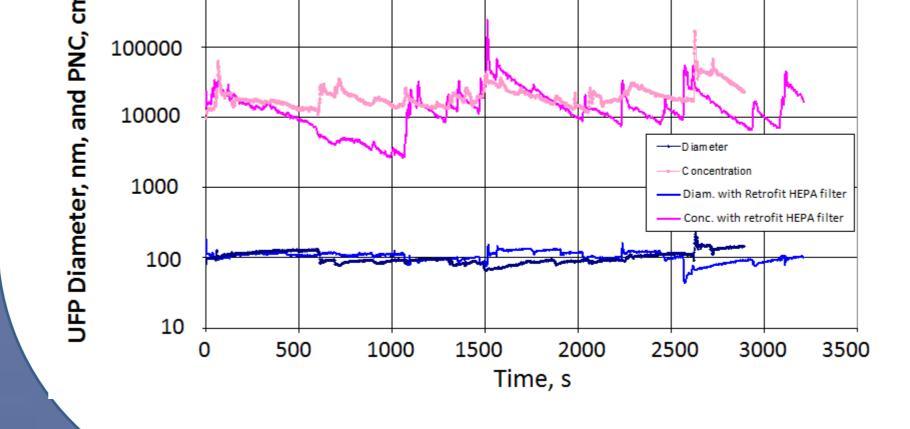
Effects of in-cabin retrofit HEPA filter, inside a shuttle taxi that frequently opens its door for passengers
