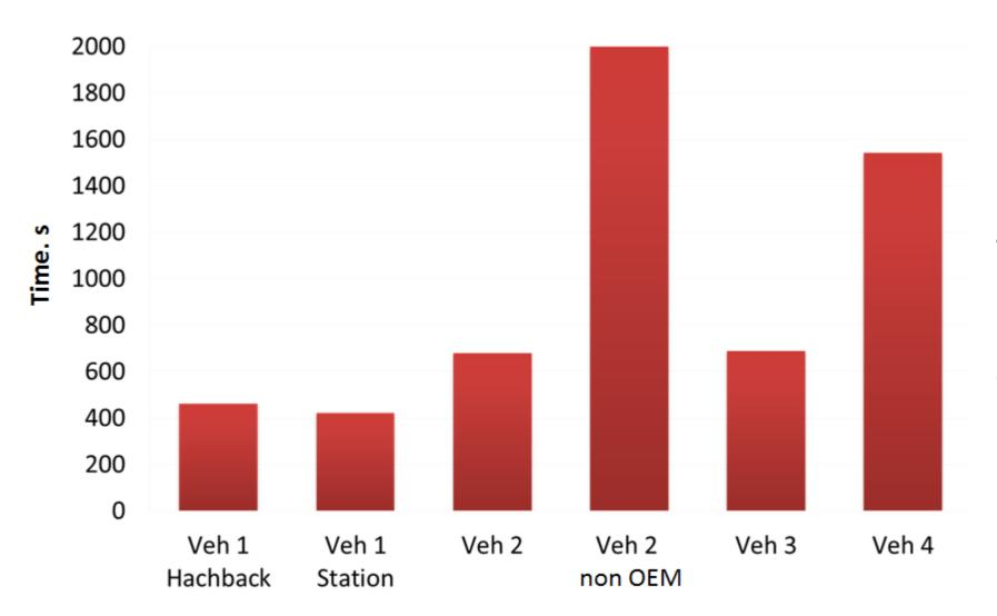
Time to reduce the concentration from 100000 to 4000 UFP per cm<sup>3</sup> for different vehicle types and sizes
