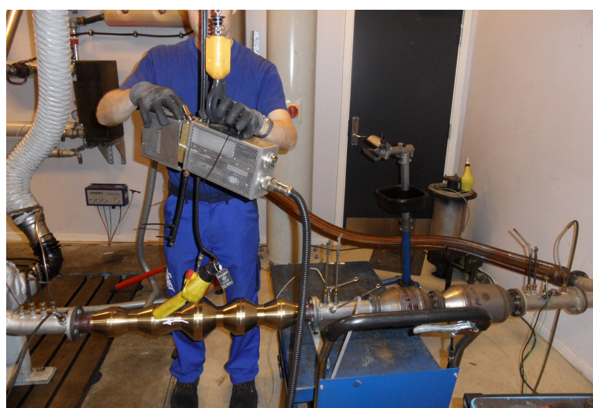
Conventional vs PAI enhanced after-treatment (EURO-III 2.5l Diesel, 1000rpm, 50Nm)
