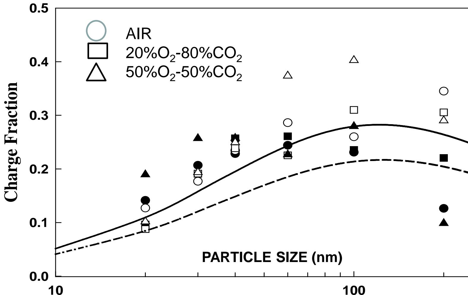
Fraction of +1 and -1 charged particles Legend: Air (-1), Air (+1), 20%O<sub>2</sub>-80%CO<sub>2</sub> (-1), 20%O<sub>2</sub>-80%CO<sub>2</sub> (+1), 50%O<sub>2</sub>-50%CO<sub>2</sub> (-1), 50%O<sub>2</sub>-50%CO<sub>2</sub> (+1).
