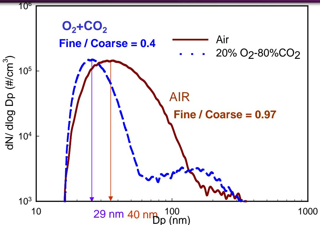
When AIR is replaced by 20%O<sub>2</sub>+80%CO<sub>2</sub>:
