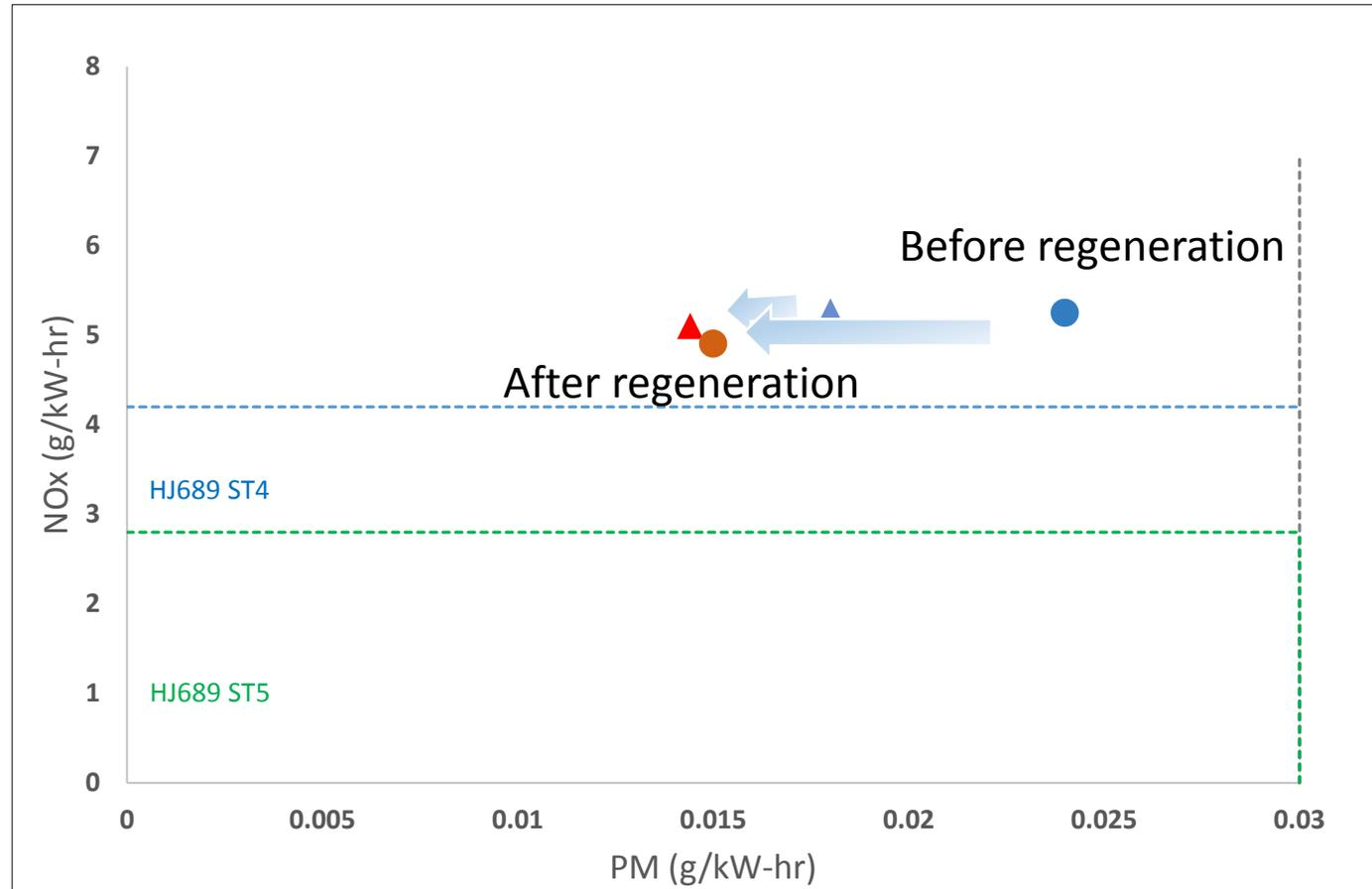
□ The efficiency of Particulate Mass reduction following regeneration were slightly higher than the brand new due to the formation of soot cake.
