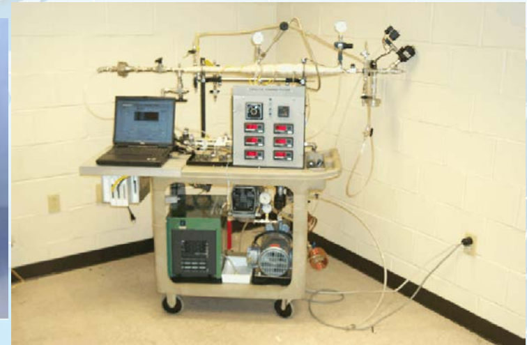
SwRI SPSS, Facilitate Solid Particle Measurement (Used Upstream of EEPS)
