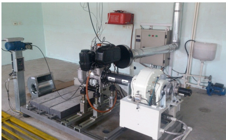
Figure 2. Engine test set up
