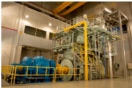
Fig. 1 Photo of Two stroke diesel engine Test bed at KR TCC (Test & Certification Center)
