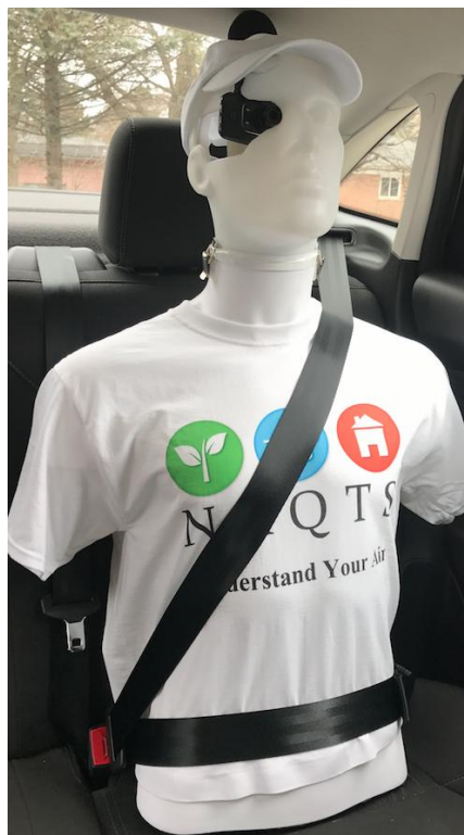
"Justin" the in cabin-air quality monitor. Can also be used for micro-environmental/mobile air quality monitoring.
