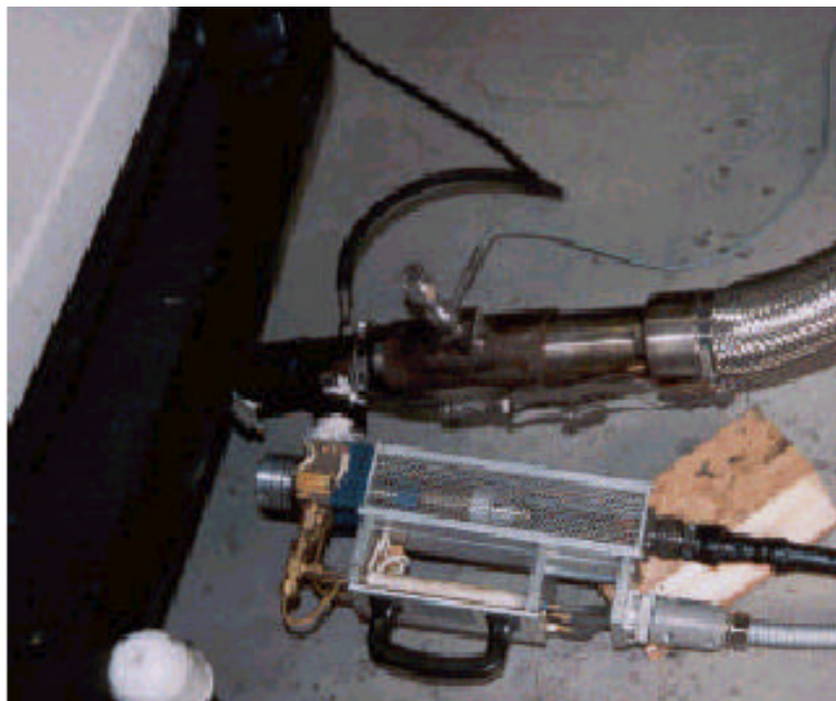
Fig. 5 Exhaust probe of rotating disk diluter to tail pipe of passenger car
