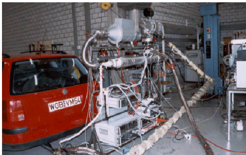
Fig. 4 VW Passat Variant with diesel engine on roller dynamometer with CVS and nanoparticle measuring systems
