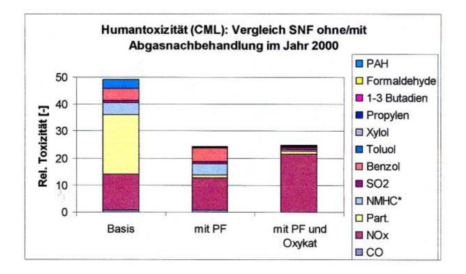
Basis: Average HDV, Year 2000, without aftertreatment Particulate trap 95% Efficiency Particulate trap + Oxidation catalyst Assumption: NO2 toxicity = 5 x NO toxicity
