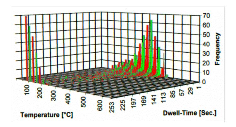
Distribution of dwell time at given temperature levels for vehicle category 2. "Frequency" here means the number of observations per temperature class (25 °C steps) and dwell time class (1 sec.-steps) with duration 1 sec per observation.
