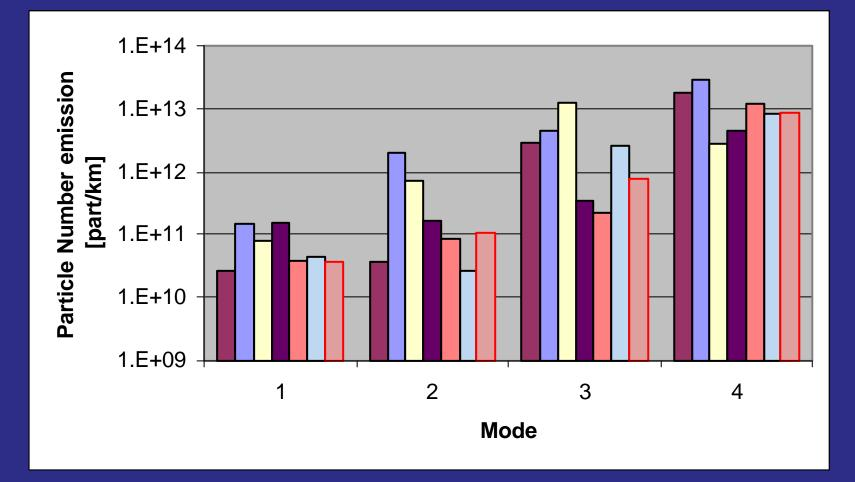
Figure 6: Particle number emissions per kilometre LPG vehicles (full bars) and ULP vehicles (patterned bars).
