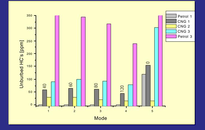
*Figure 4:* Relationship between engine speed/load and the emission levels of unburned HC's, for all five tests.
