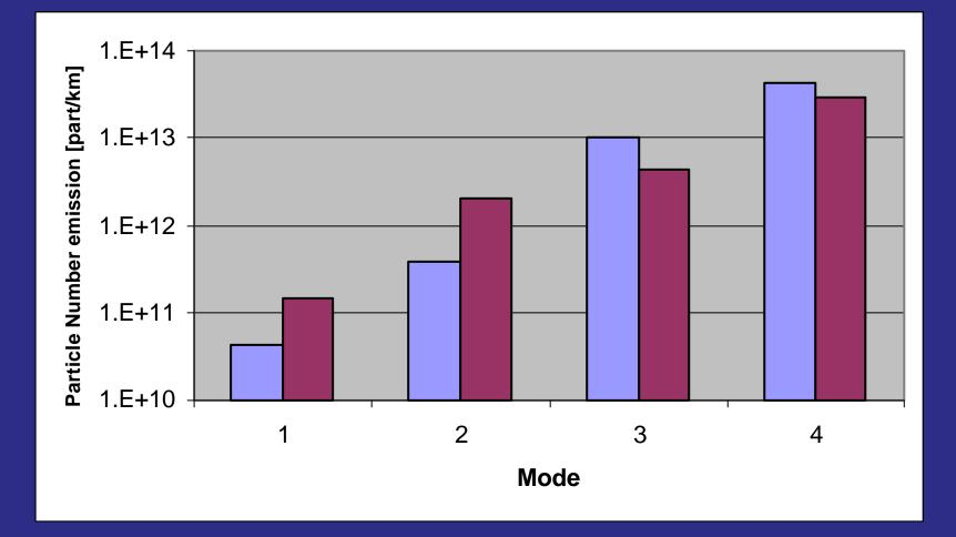
Figure 7: Particle number emissions per kilometre for the LPG vehicles 2 different tests, first test in November 2000 and second in February 2001.
