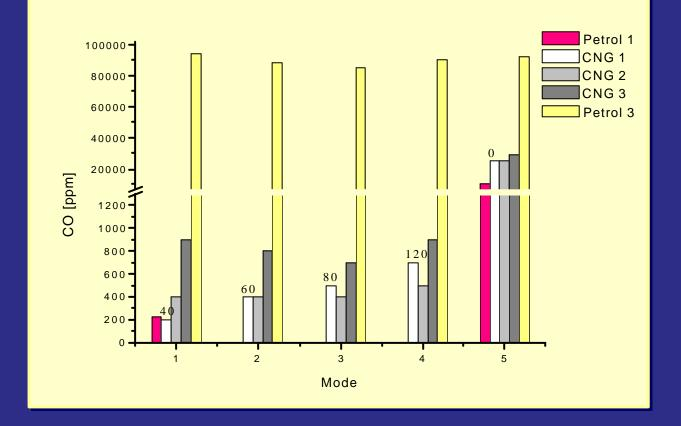
*Figure 4:* Relationship between engine speed/load and the emission levels of CO, for all five tests.
