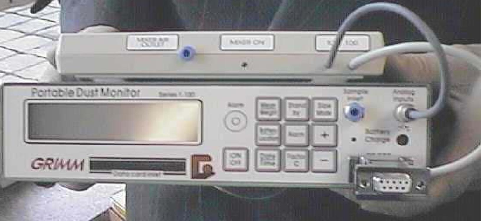
**Example of a 1.108 Laser spectrometer
