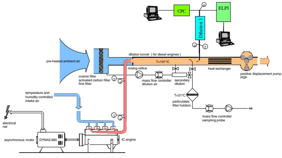
The particulate mass was determined using a state-of-the-art gravimetric filter measurement systems.
