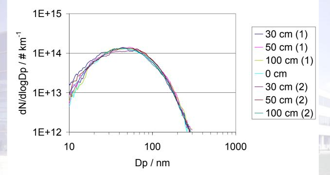
=> No influence of sampling probe extension on soot mode particles
