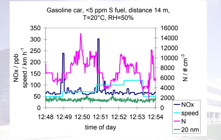
=> NO<sub>x</sub> signal detected; particles at background level
