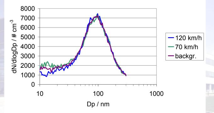
=> No soot of nucleation mode particles detected
