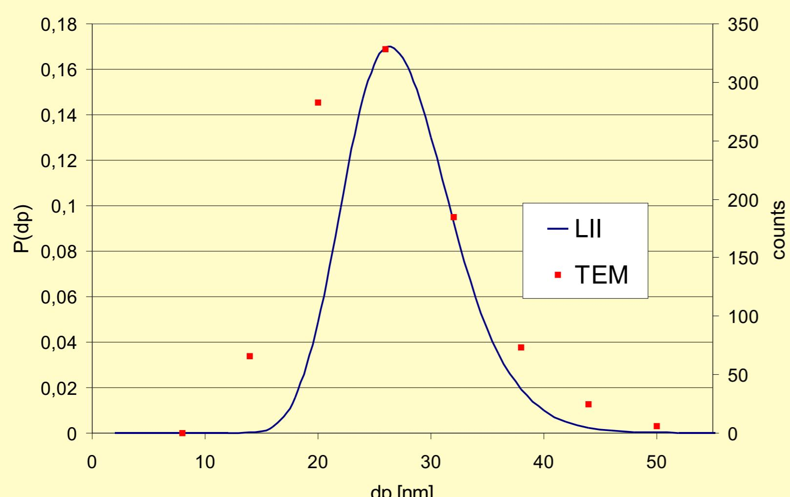
→ LI<sup>2</sup>SA is able to measure EC mass concentration (up to 20 Hz) as well as particle size distribution and mean primary particle diameter
