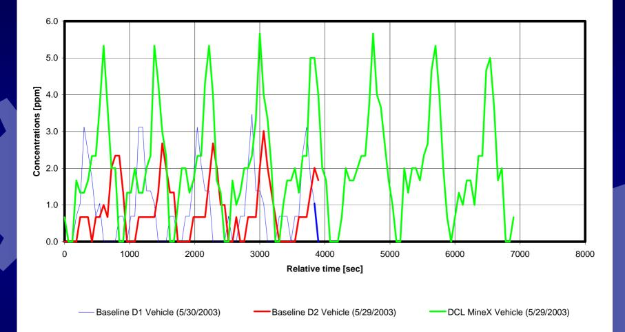
Ventilation-normalized NO<sub>2</sub> concentrations at vehicle sampling station observed during the tests with LHD #99942
