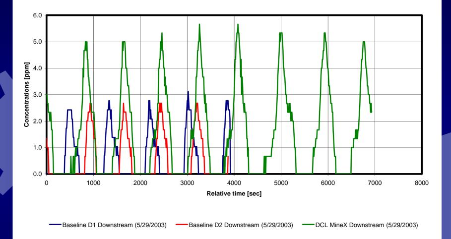
Ventilation-normalized NO<sub>2</sub> concentrations at downstream sampling station observed during the tests with LHD #99942
