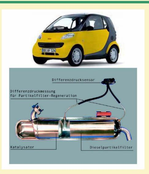
.....the application of a trap system has been demonstrated even for the smallest diesel car (DC SMART, 799 cc)
