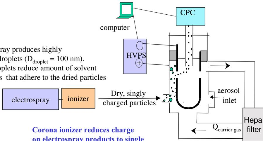
Corona ionizer reduces charge on electro spray products to single
