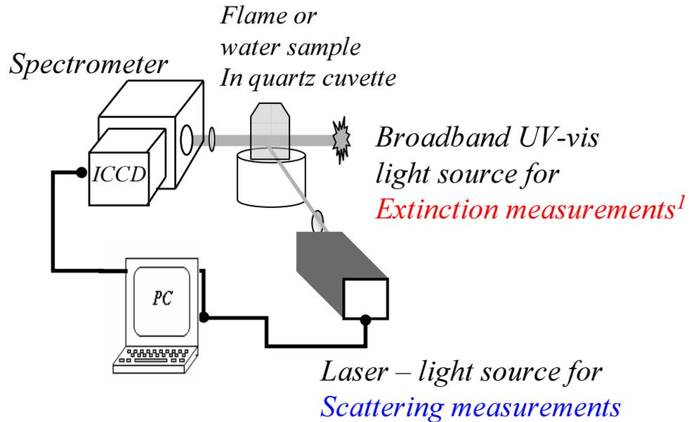
Measuring the UV-visible Extinction spectra gives the relative amounts of NOC and soot particles<sup>2</sup>
