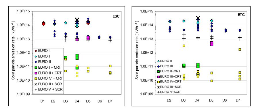
Conventional Euro-I to Euro-III engine technologies produced total solid particle number emissions in the range of 10<sup>14</sup> particles/kWh
