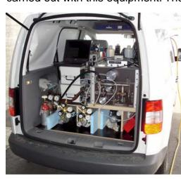
carried out with this equipment. The results allow to refer the measured ambient particle concen-trations to a common national standard and to detect hidden instabilities of the monitors.
