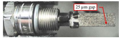
The smallest device is made of a spark plug with a very small electrode- gap to optimise the reaction time.
