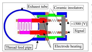
The most important part of the sensor construction consists of the electrode shaft heating. It is necessary to keep the isolation resistant within the range of 100 [M $\Omega$ ].
