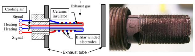
Carbon particles produce electrical resistor bridges across the electrodes and gradually reduce the isolation resistance. This principle is used as measuring device by regarding also the gradient of the resistor changing as a measure of the dynamic particulate concentration. The bifilar coil is manufactured of resistance material and by simply shorten the ends of the coils the measuring device is used as well for burning the particulates.
