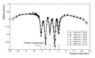
The exhaust tube of 50 [mm] diameter was scanned across for a range of engine speeds and engine loads. The measured results had to be normalized in order to see the profile at different gas flow speeds. Even at the positions of the electrode blades inside the tube the profile stays constant. This is the necessary condition for on board measurements of high accuracy.
