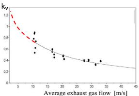
The gas flow speed has to be derived from the air intake mass flow, the fuel mass flow, the exhaust tube diameter and the temperature at the sensor position.
