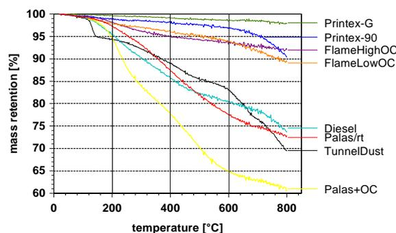
Fig. 1 Thermogravimetry shows the mass decrease during gradual heating in a nitrogen gas flow.
