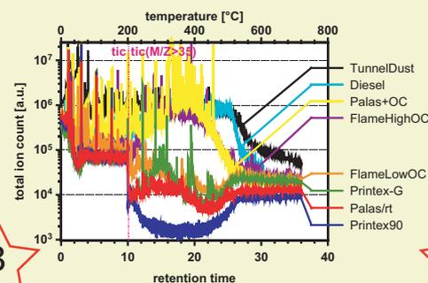
PyrGC-MS distinguishes between high and low OC samples at temperatures over 200 °C. For better resolution, components of M/Z < 35 are neglected after 10' retention time
