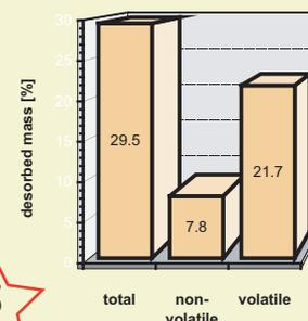
The desorbed matter does not consist gaseous components only. The gas flow from Palas/rt sample was filtered using a gold sputtered nuclepore filter. We found 7.8 % of the sample mass on it. EDX analysis of the particles on the filter give evidence for carbonaceous particles.
