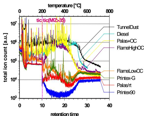
Fig. 2 Ion counts of GC-MS. Temperature rises with 20 K/min. To gain resolution, at 10 minutes retention time, all counts below  $M/Z=35$  are neglected.
