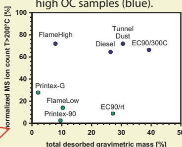
Organics are known to volatilize above 200 °C. The ratio of the MS-ion-count for temperatures above 200 °C normalized by the total ion count separates high OC from low OC samples.
