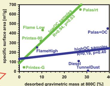
Desorbed gravimetric mass correlates well with BET specific surface area for the low OC samples (green). No correlation is found for high OC samples (blue).
