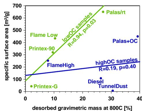
Fig. 4 Desorbed gravimetric mass correlates well with BET specific surface area for the low OC samples (green). No correlation is found for high OC samples (blue).
