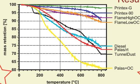
Thermogravimetry shows the mass decrease during gradual heating in nitrogen.
