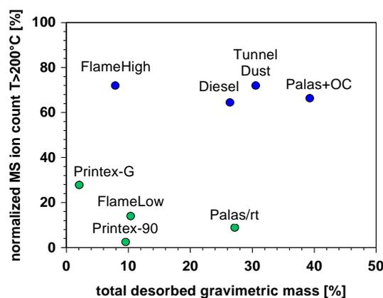
Fig. 3 Desorbed gravimetric mass and integrated normalized total ion count of mass spectrometry for retention time 10 ... 36 min.
