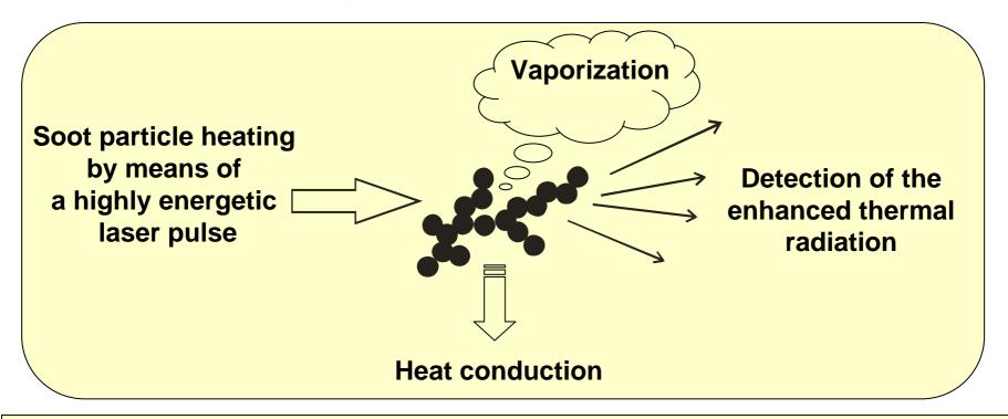
$$\underbrace{Q_{abs} \cdot \frac{\pi d_p^2}{4} \cdot E_i}_{Absorption} - \underbrace{\Lambda \cdot (T - T_0) \cdot \pi d_p^2}_{Heat \ conduction} + \underbrace{\frac{\Delta H_S}{M} \cdot \frac{dm}{dt}}_{Vaporization} - \underbrace{\pi d_p^2 \int \mathcal{E}(d_p, \lambda) M_\lambda^b(T, \lambda) \cdot d\lambda}_{Thermal \ radiation} - \underbrace{\frac{\pi d_p^3}{6} \rho_S \cdot C_S \cdot \frac{dT}{dt}}_{Change \ of \ internal \ energy} = 0$$
