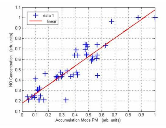
With auto-ignition (HCCI), residuals improve mixture preparation, but decrease oxidation in the expansion stroke. Burn rates are not diffusion limited PM scales with load, rather than with EGR.
