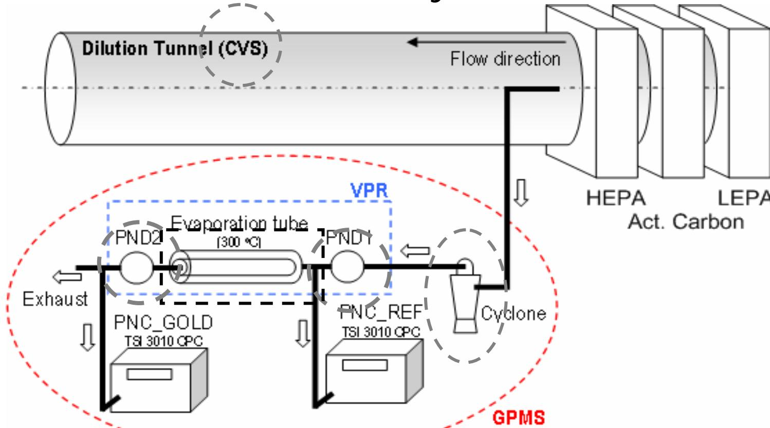
A particle number method employing a condensation nucleus counter, but using sample pre-conditioning to eliminate the most volatile particles which may contribute significantly to variability.
