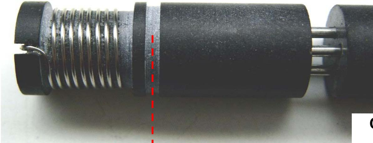
Cleaned sensor after 2 days operation
