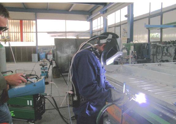
Figure 2: Hand-held measurement of UFA in a welding-shop to evaluate the effectiveness of personal respiratory protection.
