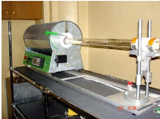
Figure 2. Thermal shock test bench.
