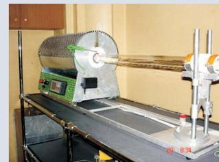
Figure 8. Thermal shock test bench.
