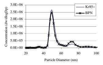
Figure 2 Example size distributions measured when passing a mono-disperse aerosol (50 nm) through either a radioactive ( $Kr^{85+}$ ) or electrical neutralizer.
