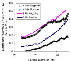
Fig. 3: Comparison of charge per particle vs particle diameter for the Kr85+ source and the BPN.
