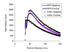
Fig. 2: Size Distributions as measured using the radioactive and electrical neutralizers with the DMA scanning both positive and negative high voltages.
