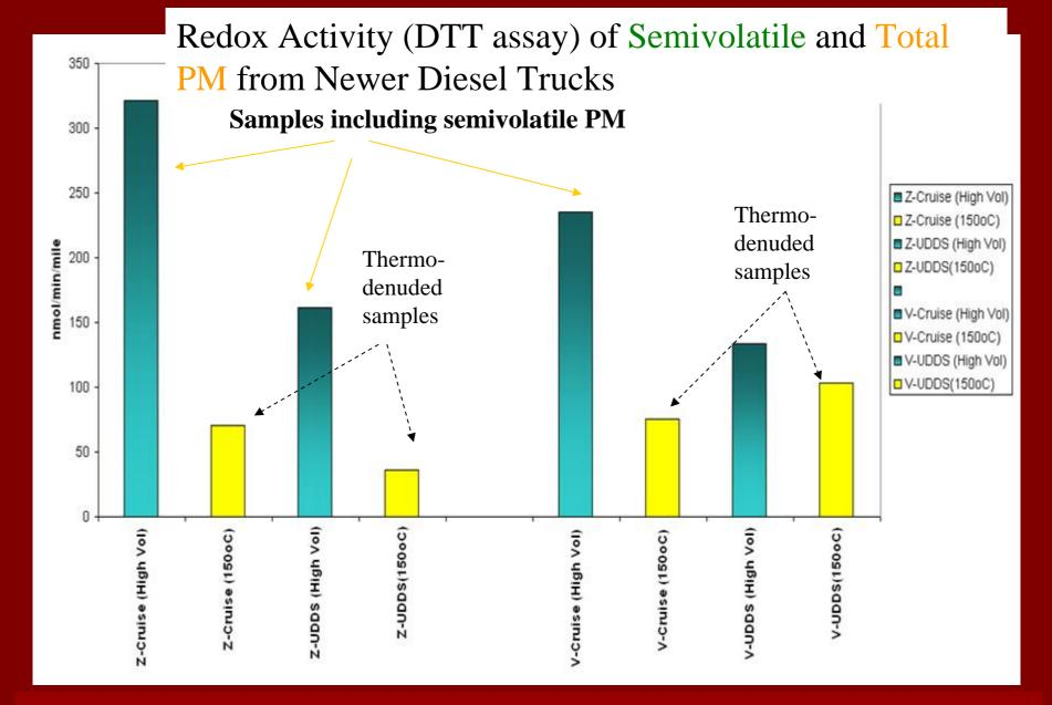
DTT rate of consumption per PM mass (nmoles/µg PM/min) is <u>much</u> <u>higher when the semi-volatile fraction is included</u>
