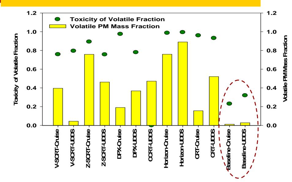
Toxicity of volatile fraction= [(DTT,Undenuded, n-mole/km/min) - (DTT at150oC, n-mole/km/min)] / [DTT ,Undenuded, n-mole/km/min)]
