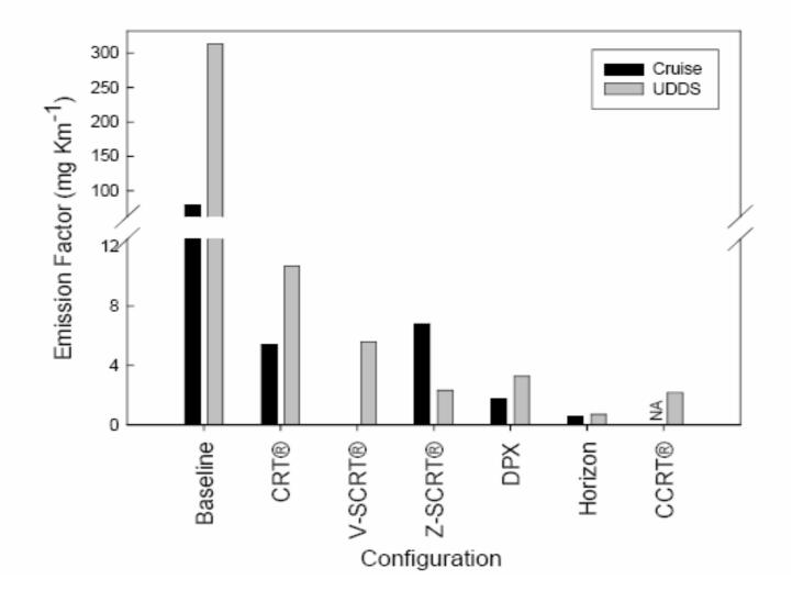
Mass PM emission rates for baseline vehicle are 20- 100 times higher than those of the rest of the tested fleet
