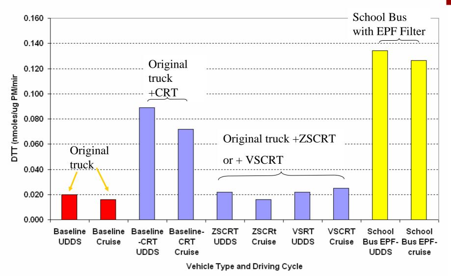
DTT activity expressed <u>per PM mass</u>; note the very high activity of some of the reduced mass emission trucks, especially with <u>non-catalyzed silicon carbide</u> (CRT) substrate for PM control
