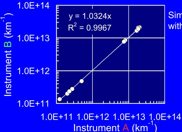
Simultaneous sampling with instrument A and B
