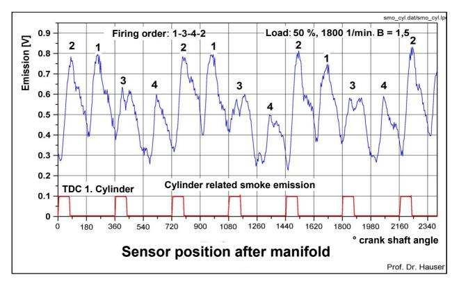
It must be mentioned that, without knowing the exhaust gas speed, no calibrated measurement is possible. Therefore a software was designed to adapt these results on-line to a stationary operating soot measuring instrument. After this stationary procedure high speed soot measurements with a rise time of 10 [ms] can be achieved.
