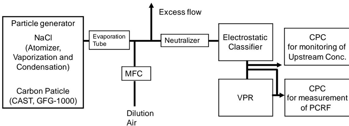
Figure 5 Experimental setup for measurement of Particle Concentration Reduction Factor
