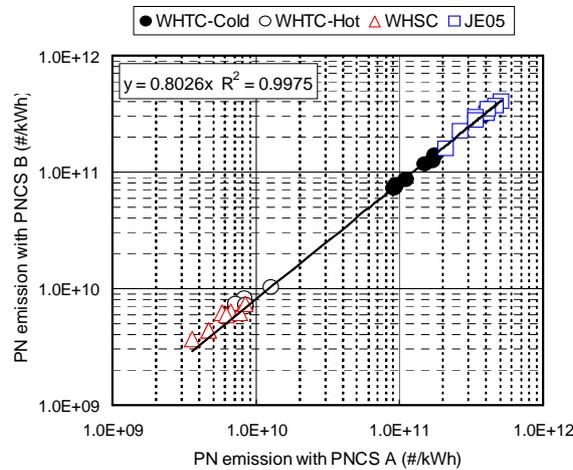
Figure 4 Particle number emissions from J08E-TP with two types of PNCS
