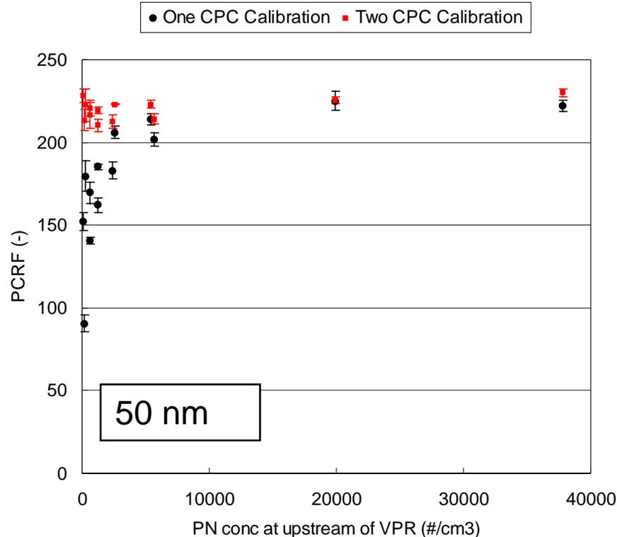
PCRf measurements were influenced by inlet conc. of VPR with one CPC calibration.
