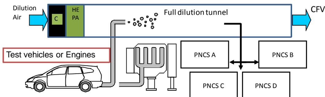
Figure 1 Experimental setup for simultaneous measurement of PNCS
