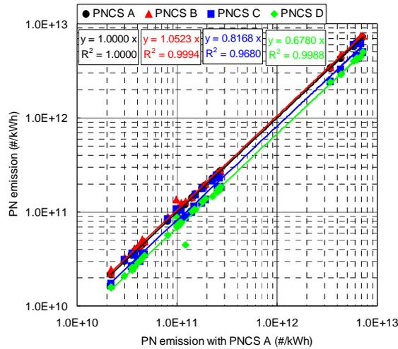
Figure 3 Particle number emissions from OM501 with four types of PNCS
