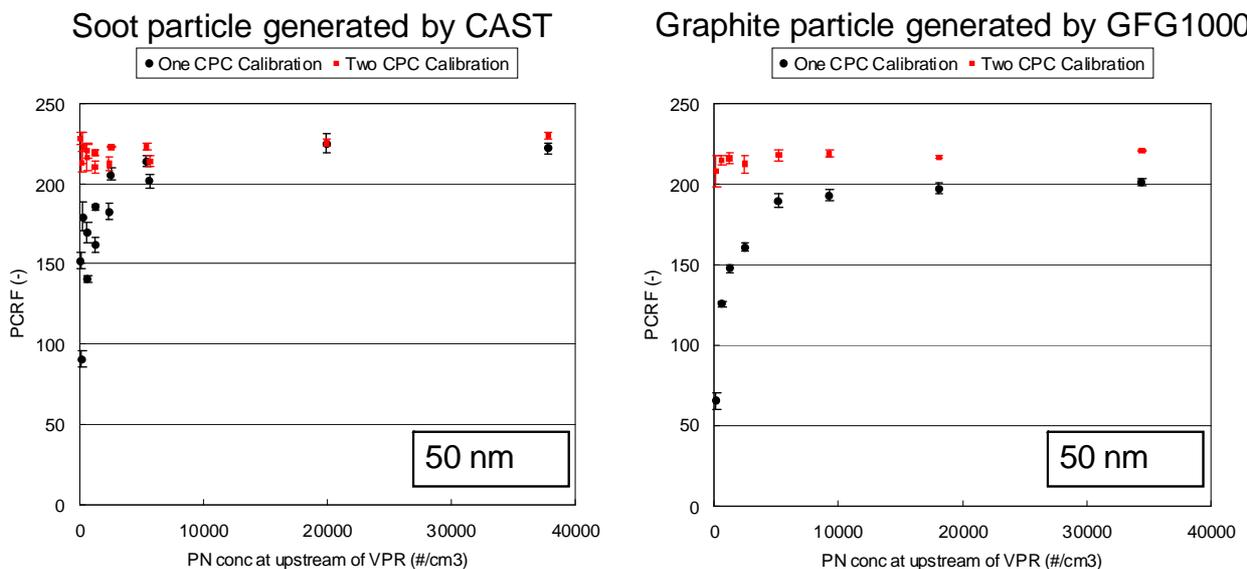
Figure 7 Relationships between PCRf and particle concentration at upstream of the VPR
