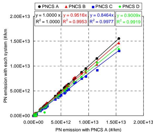
Figure 2 Particle number emissions from vehicles with four types of PNCS
