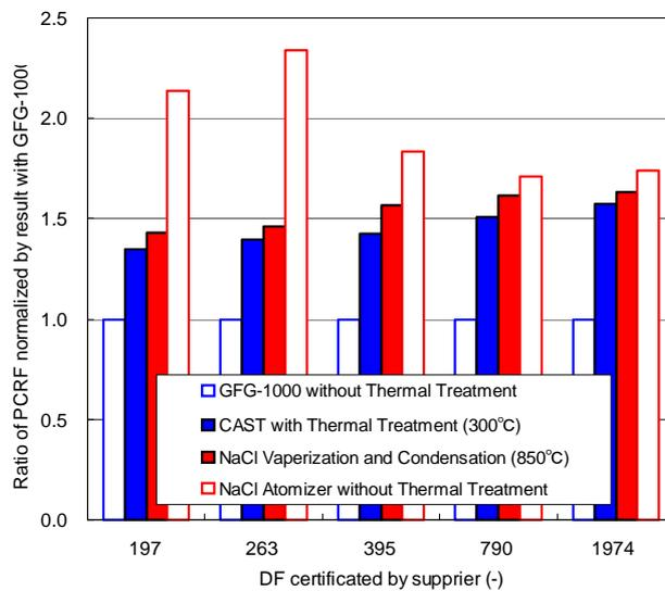
Figure 10 Ratio of PCRf with several particles to that with GFG-1000
