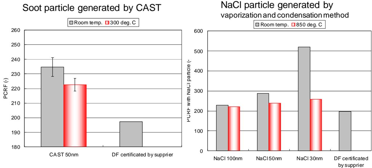
Figure 6 Influence of thermal treatment of generated particle on PCRf measurement
